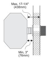
For straight rear installation, Restrictor must be set at 1-1/8" open.
